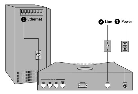
1. Connect one of the RJ-45 cables to any of the Ethernet ports on the router.
